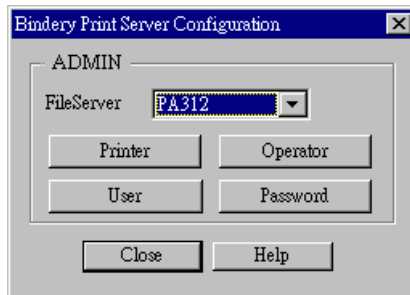
Figure 14: Configure NetWare Server (Bindery PS mode)
