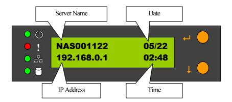
At this time the hardware installation of your LevelOne NAS is complete. Please proceed to "Set-up before First Operation".
