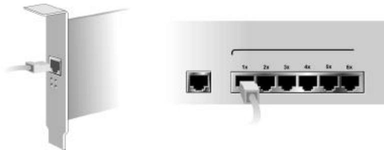
*Figure 2.3 Connecting Workstations*
