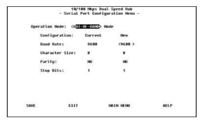
Figure 5.10 Out-of-band Operation Mode
