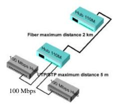
Figure 2.5 Connecting Fast Ethernet Hubs
