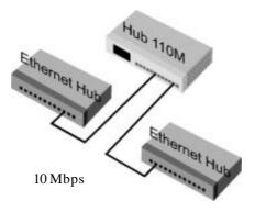
Figure 2.4 Connecting Ethernet Hubs
