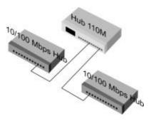
Figure 2.6 Connecting the Other Dual Speed Hubs
