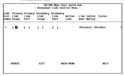
Figure 5.22 Configuring Redundant Link Control
