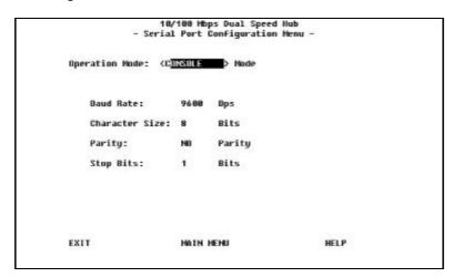
Figure 5.9 Console Operation Mode
