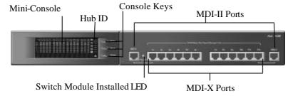
Figure 1.10 Front Panel Hub FHU-1202TFXS (12 Port)
