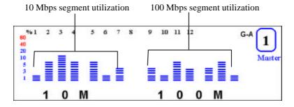
Figure 4.3 Utilization per Segment
