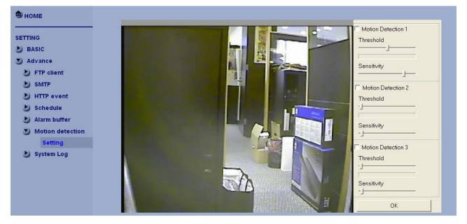
Click it On when you use the Motion Detection function and detecting zone appears for adjusting and moving. The common setting options are displayed below. If you do not wish to use the Motion Detection function, click it Off and press OK.
