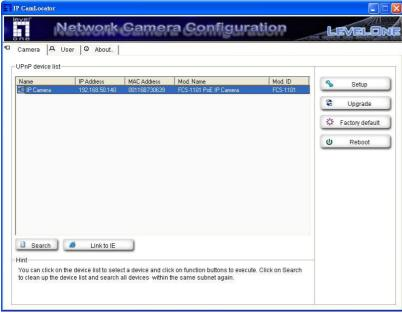
The IP addresses shown in the "IP Address" field reflect those on the local network. They may be from the DHCP server. If there is no DHCP server, the camera will try to find a free IP address (this takes from 15 second to 3 minutes, depending on the LAN status). The method of finding IP address is seeking from 192.168.0.2, to 192.168.0.254. If any of the address inside this range is free, the Network Camera will be assigned to this IP address, and its subnet mask would be 255.255.255.0.
