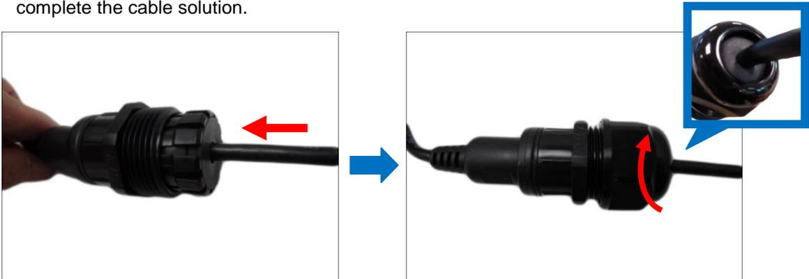
**NOTE:** Make sure the clamping nut is tightly attached to the cable gland body and the sealing insert is squeezed tightly.
