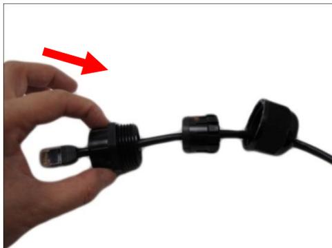
5. On the "pigtail" side, insert the washer into the "pigtail".
