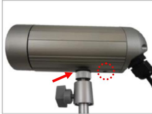
3. Adjust the camera viewing angle and tighten the knob to fix the camera position.
