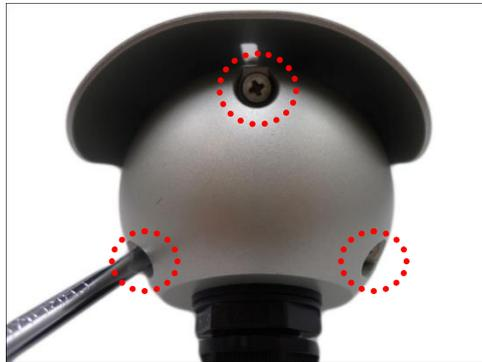
**NOTE:** A cable is connected inside the camera; do not abruptly pull the back cover.
