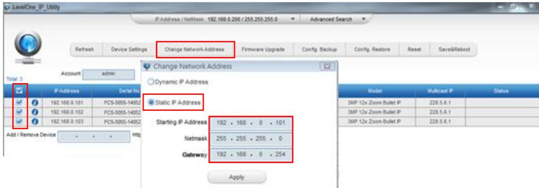
With the procedure shown above, all the cameras will have unique IP addresses, starting from 192.168.0.101. In case there are 20 cameras selected, the last one of the cameras would have the IP 192.168.0.120.
