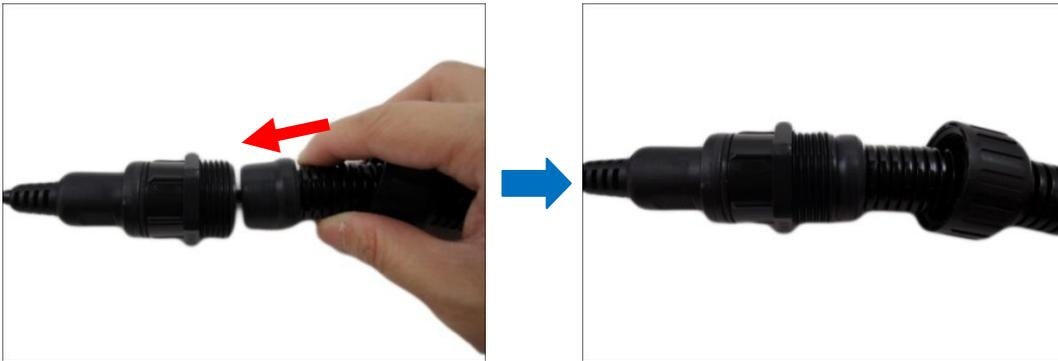
**NOTE:** Make sure the clamping nut is tightly attached to the cable gland body and the sealing insert is squeezed tightly.
