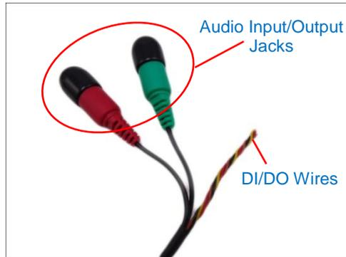
**NOTE:** If these connectors will not be used, leave the rubber caps on and the wires twisted together to ensure cables remain waterproof and eliminate short-circuit hazards.
