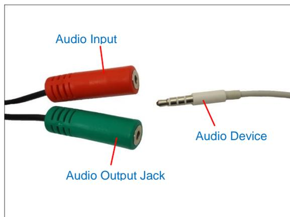
**Note:** Make sure that the connected audio input device has a built-in amplifier. Connecting an ordinary microphone will dwarf sounds and will result in inaudible recording.
