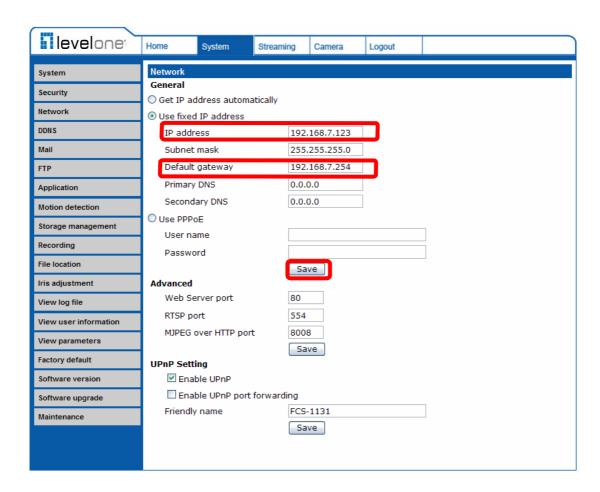
When using static IP address to login to the IP Camera, users can access it either through "DeviceSearch" software (see <u>"Accessing Camera"</u>) or input the IP address in the URL bar and press "Enter".
