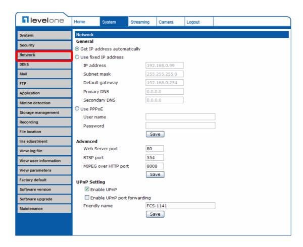
Users can choose to connect to the IP Camera with fixed or dynamic (DHCP) IP address. The IP Camera also provides PPPoE support for users who connect to the network via PPP over Ethernet (PPPoE).
