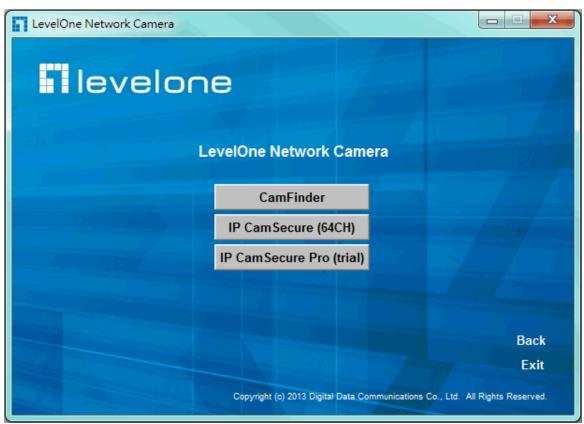
"Cam Finder" is used to search the IP address of Network Cameras or Video servers on a LAN. After searching, Video Servers or Network Cameras will be located by the Cam Finder.
