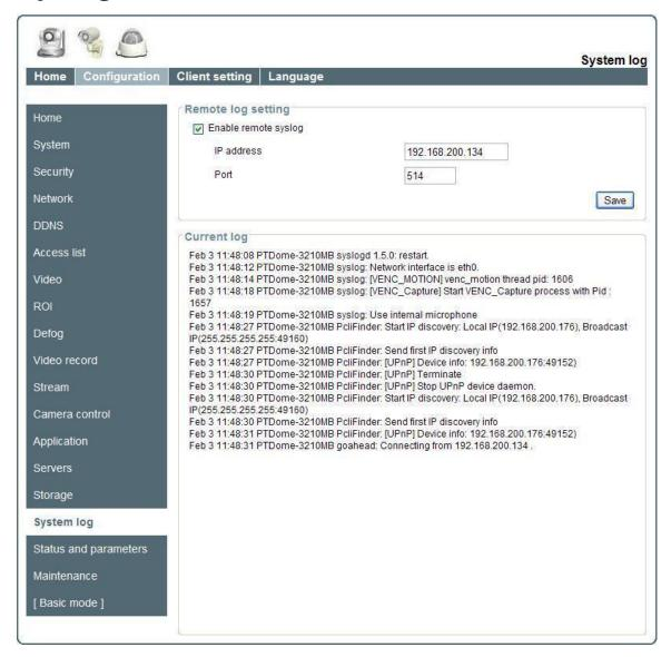
You can configure the Network Camera to send the system log file to a remote server as a log backup. Before utilizing this feature, it is suggested that the user install a log-recording tool to receive system log messages from the Network Camera. An example is Kiwi Syslog Daemon.
