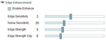
Check the box **Enable** to enable this function. There are 4 slide bars for adjustment. The **Edge Sensitivity** represents how textures are detected as edges. The higher **Noise Sensitivity** value makes noises to be filtered out, and avoid to amplify noises. The **Edge Strength** is a capability to enhance edges with a limitation by **Edge Strength Clip** to avoid over artificial edges.
