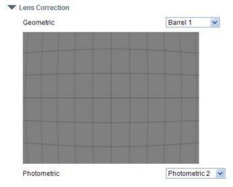
Geometric lens correction is used to correct lens distortion. The lens distortion includes barrel distortion and pincushion distortion if a lens is wide angle view or telescope, respectively.
