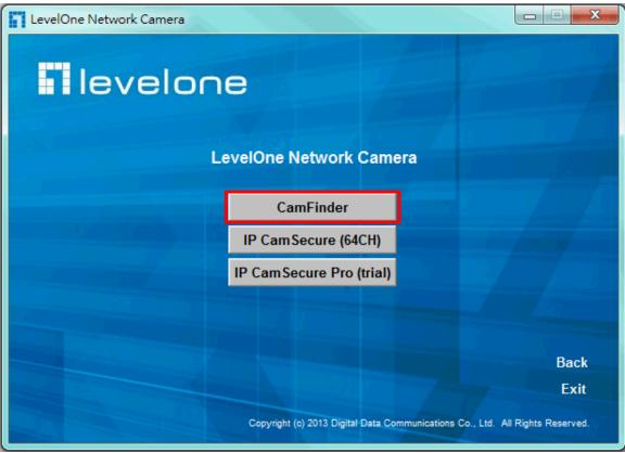
"IP Finder" is used to search the IP address of Network Cameras or Video servers on a LAN. After searching, Video Servers or Network Cameras will be located by the IP Finder.
