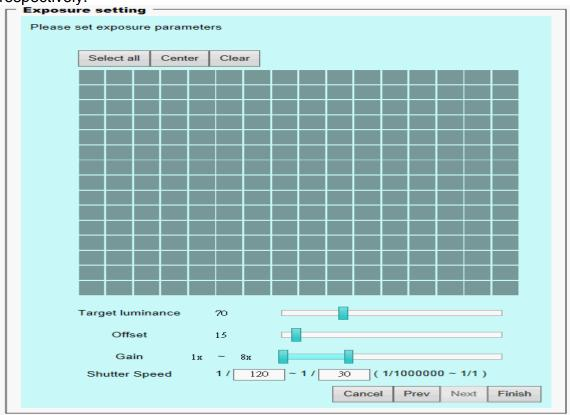
**Customized** mode relates to the grid window above can be pointed on for interesting areas. Within the mode Customized, 16\*15 grids windows can be chosen to match where/what you are interested in. Push down left-button of mouse and drag to draw the grids for interesting areas, or push down right-button of mouse and drag to clean the grids for insignificant areas.
