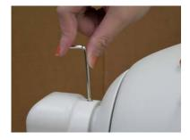
unscrew the bottom screw to install cables.
