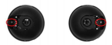
◆ Finally cover up the smoked cover to accomplish the installation. Please be sure hands are clean while cover up, or it may dirty the cover. It's recommended to tear off the protect membrane after installation is finished, or wear on gloves.
