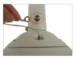
4. Align the bigger end of the safety wire strap on the mounting solution and then tightly attach the screw to lock the safety wire strap in place.
