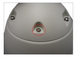
2. Insert the screw through the smaller end of the safety wire strap and attach it to the camera.
