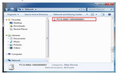
Double-click the mouse on the camera model name, the default browser of the PC is automatically launched and the IP address of the target camera is already filled in the address bar of the browser.
