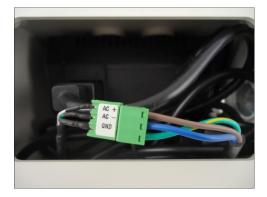
d. Install a female power socket (not included) inside the junction box to plug the cord and power up the camera.
