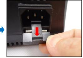
2. Remove the main fuse from its bay and pull to retrieve the replacement fuse.
