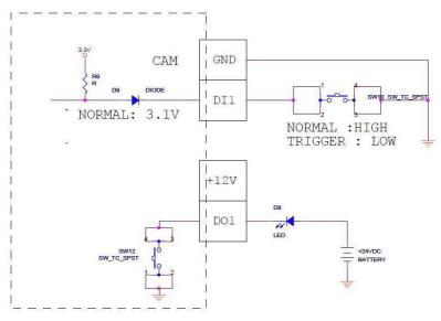
Consequently, to connect a second DI or DO device, use the Black (GND) and Green (DI2) cables to connect the second DI device, and the Red (12V) and Blue (DO2) cables for the second DO device.
