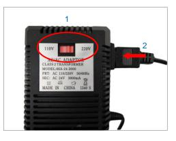
3. Connect the power connector of the camera to the cable connector of the adapter.
