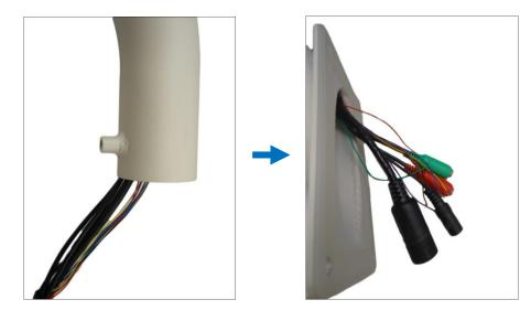
CAUTION: The camera itself is waterproof, however take note that the cable connections are not. If the cable connections will be exposed outdoors, make sure to shield or adapt proper waterproofing methods. See *Step 3: Waterproof the Cable Connections* on page 16.
