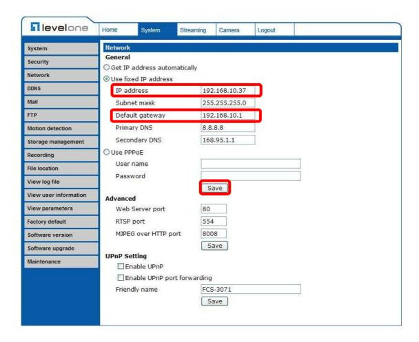
When using static IP address to login to the IP Camera, users can access it either through "Device Search" software (see :Accessing Camera") or input the IP address in the URL bar and press "Enter".
