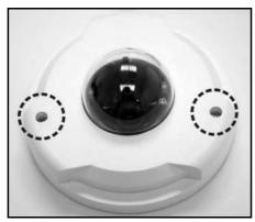
**Step 2:** Loosen the focus fixed screw, and rotate the lens counter-/clockwise to adjust focus; loosen the tilt fixed screw, and adjust the camera's tilt angle.
