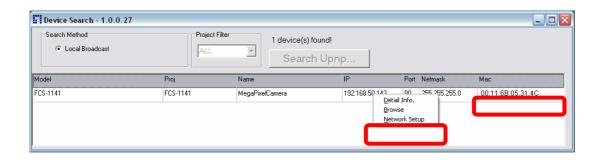
**Step 2:** The "Network Setup" page will come out. Select "DHCP," and press "Apply" button down the page.
