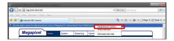
Then the security warning window will pop up. Click "Install" to carry on software installation.
