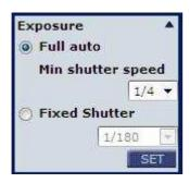
The exposure is the amount of light received by the image sensor and is determined by the width of lens diaphragm opening, the amount of exposure by the sensor (shutter speed) and other exposure parameters. With this item, users can define how the Auto Exposure function works.
