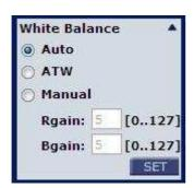
A camera needs to find reference color temperature, which is a way of measuring the quality of a light source, for calculating all the other colors. The unit for measuring this ratio is in degree Kelvin (K). Users can select one of the White Balance Control modes according to the operating environment. The following table shows the color temperature of some light sources for reference.
