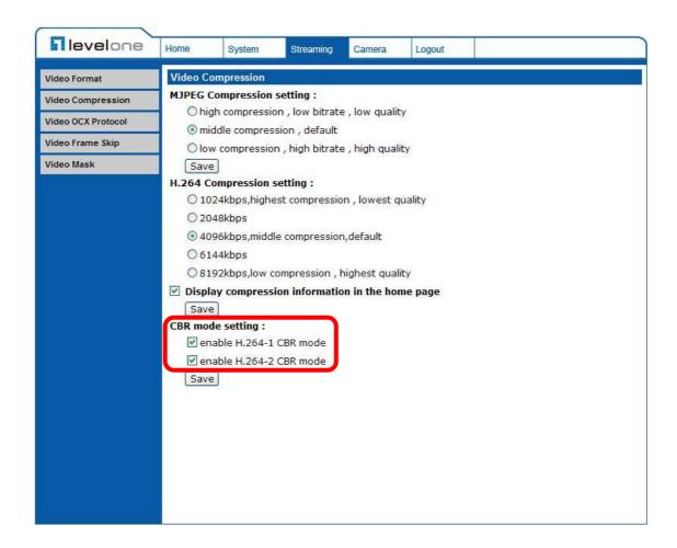
The CBR (Constant Bit Rate) mode could be the preferred bit rage mode if the bandwidth available is limited. It is important to take account of image quality while choosing to use CBR mode.
