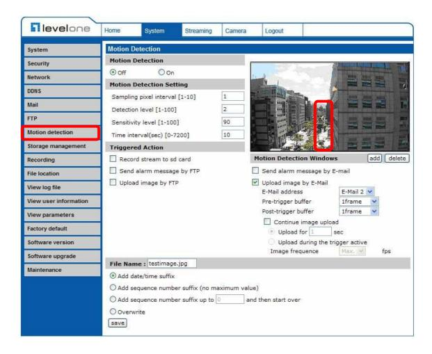
In the Motion Detection setting page, there is a frame (**Motion Detection Window**) displayed on the Live View Pane. The Motion Detection Window is for defining the motion detection area. To change the size of the Motion Detection Window, move the mouse cursor to the edge of the frame and draw it outward/inward. Moving the mouse to the center of the frame can shift the frame to the intended location.
