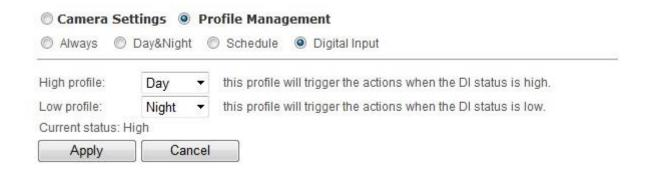
**Digital Inputs -** Select Digital Input to have the profile management controlled by an external sensor. Select profiles from the drop down menu. Profiles will change according to different trigger voltage levels.
