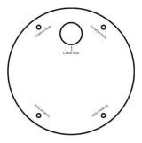
iii. Hammer the four plastic anchors which are provided in the product package into the four location holes.
