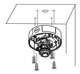
WARNING: Do not mount the camera on a soft material. The camera may fall and be damaged.
