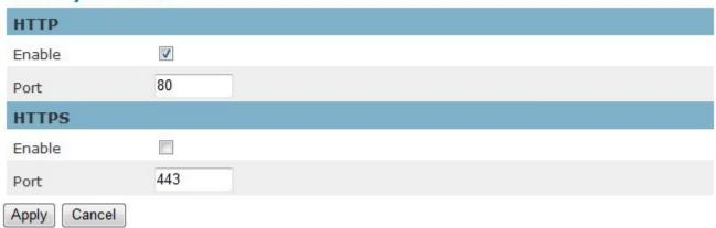
**HTTP** – (Hypertext Transfer Protocol) - This protocol allows for TCP protocol quality without having to open specific ports for streaming. Users inside a firewall can utilize this protocol to allow streaming data through.
