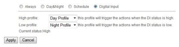
**Digital Input -** Select Digital Input to have the profile management controlled by an external sensor. Select profiles from the drop down menu. Profiles will change according to different trigger voltage levels.
