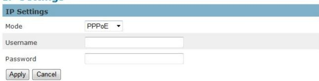
3. **PPPoE** (Point-to-point over Ethernet): Use this mode if connecting to the Internet through a DSL Line. **NOTE** - To utilize this feature, it requires an account provided by an Internet Service Provider. Enter the user name and password provided by the ISP.
