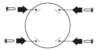
iv. Mount the camera on the wall and position the four screw slots over the plastic anchors. Insert the screws into the holes and use the screwdriver to tighten the screws clockwise until they are secure.
