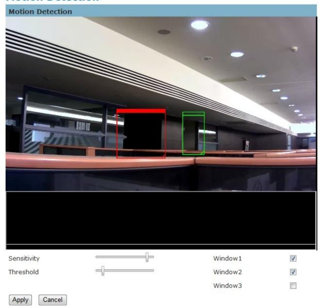
**Detection Setting –** Use this setting to enable and define the motion detection windows. The user can defined up to three areas on the live view window for motion detection.
