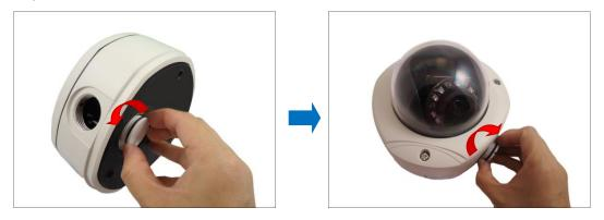
2. Loosen the three (3) screws securing the dome cover.
