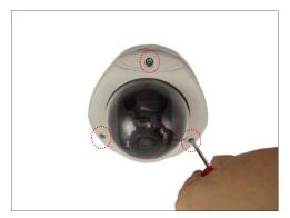
3. Remove the plastic covering the dome cover. Final installation will look like the illustration below.
