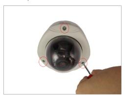
2. Using a screwdriver, remove the screw securing the spring wire to the dome cover.
