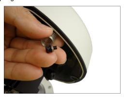
10. Attach the screw to the dome cover using a screwdriver. Final installation should look like the illustration below.
