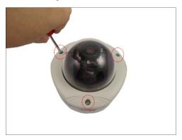
3. Carefully lift to open the dome cover and place it on the side of the camera.
