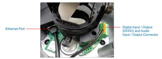
3. Connect the other end of the network cable to a switch or injector. Then, connect the switch or injector to a network or PC and a power source. See Power-over-Ethernet (PoE) example connection diagram below.
