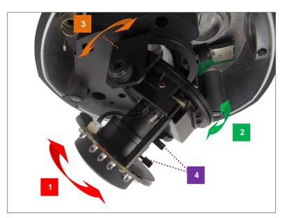
1. Loosen the tilt adjustment screws, adjust the tilt, and then tighten back the screws to fix the tilt position.
