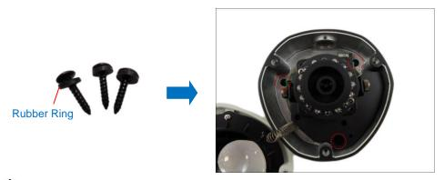
CAUTION: When using electric screwdrivers, be careful not to touch the internal camera components while attaching the screws. Since electric screwdrivers vary in sizes, speed, and force, they may bruise and damage the internal camera components.
