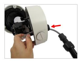
b. Insert the sealing nut into the conduit gland body and then attach the clamping nut to complete the cable solution.
