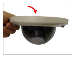
8. Align and attach the three (3) screws to secure the bracket to the cover housing.
