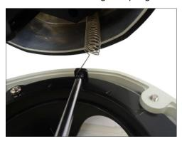
**NOTE:** Hold the spring wire as the screw is being removed to avoid the sudden release of the screw and cause it to fly in the air.
