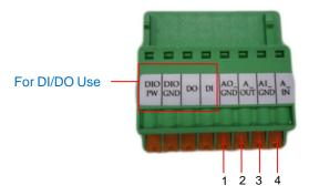
To connect audio devices, map the pins to one of the pin combinations below:
