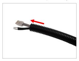
4. Insert the clamping nut through the flex conduit.
