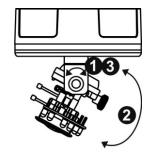
iii. Release the video adjustment screw and to adjust the lens direction. After completion, tighten the video adjustment screw.
