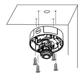
**!** WARNING: Do not mount the camera on a soft material. The camera may fall and be damaged.
