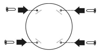
iv. Mount the camera on the wall and position the four screw slots over the plastic anchors. Insert the screws into the holes and use the screwdriver to tighten the screws clockwise until they are secure.
