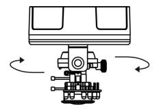
ii. Release the tilt screw on both side of the device to rotate the lens up or down. After completion, tighten the tilt screw.
