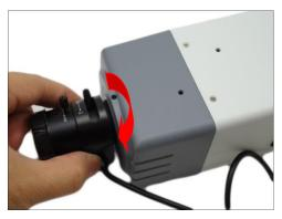
4. For lens with DC-iris, connect the lens cable to the DC-iris port of the camera.
