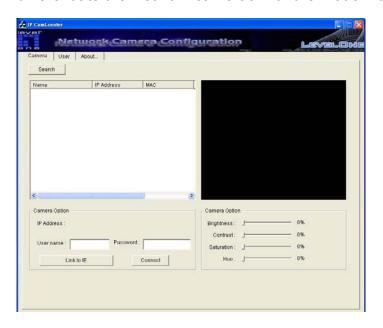
The IP addresses shown in the "IP Address" field reflect those on the local network. They may be from the DHCP server. If there is no DHCP server, the camera will try to find a free IP address (this takes from 15 second to 3 minutes, depending on the LAN status). The method of finding IP address is seeking from 192.168.0.2, to 192.168.0.254. If any of the address inside this range is free, the Network Camera will be assigned to this IP address, and its subnet mask would be 255.255.255.0.
