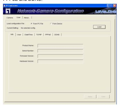
**Load configuration File**: Select **From PC File** or **From Device**, the former one can load information of downloaded configuration file and the latter one can load Network Camera configurations in the network.
