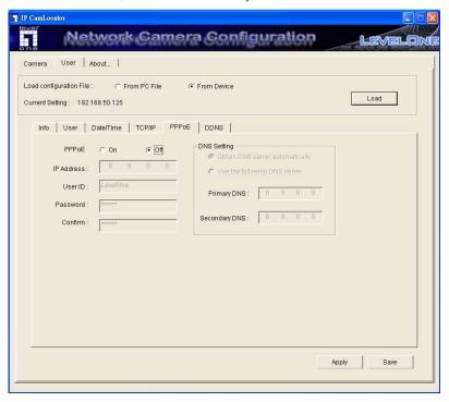
**IP Address**: The IP address obtained at the PPPoE connecting with network.
