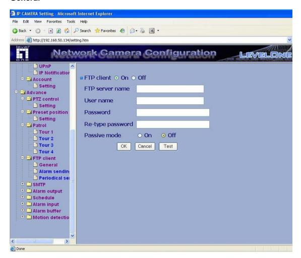
**FTP client function**: To activate the FTP client function, select **On**. The FTP client setting page appears. When you do not wish to use the FTP client function, select **Off**. *Note:*
