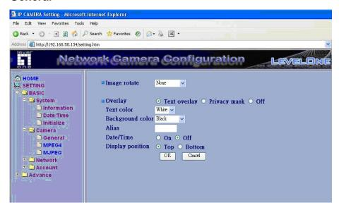
Image Rotate: Select to Mirror, Rotate, or Mirror & Rotate the display image.
