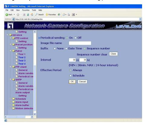
**Image file name**: Type the file name of the image sent by SMTP up to 10 alphanumeric characters, - (hyphen) and \_ (under score).
