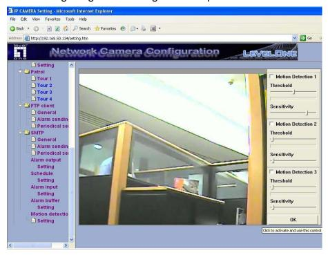
Click it **On** when you use the Motion Detection function and detecting zone appears for adjusting and moving. The common setting options are displayed below. If you do not wish to use the Motion Detection function, click it **Off** and press **OK**.
