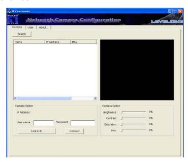
**Search**: Click it to search network cameras in the network, it displays network cameras information including product name, IP address, MAC address, model name and model ID. **Link to IE**: After searching network cameras in network, you can click to specific Network cameras in search area and press **Link to IE** to set the video server of the network camera in Microsoft web browses.
