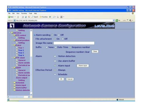
**Alarm sending**: Select **On** to set to send mail with connection to the alarm detection.
