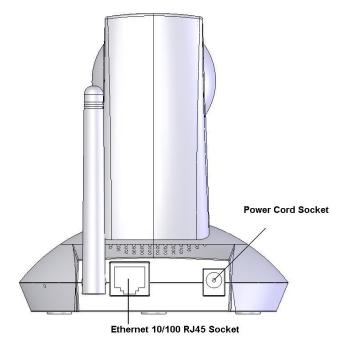
Connect the power adapter jack to the Network Camera before plugging in to the power socket. This will reduce the risk of accidental electric shock.
