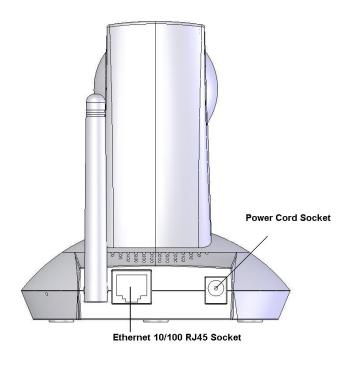
Connect the power adapter jack to the Network Camera before plugging in to the power socket. This will reduce the risk of accidental electric shock.
