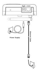
Connect the power adapter jack to the Network Camera before plugging in to the power socket. This will reduce the risk of accidental electric shock.
