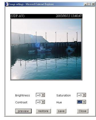
ranged from -5 to +5. In **"Brightness"** and **"Contrast"** fields the value 0 indicates auto tuning. The user may press <u>Preview</u> to fine-tune the image. When the image is O.K., press <u>Save</u> to set the image settings. <u>Restore</u> Click on this to recall the original settings without incorporating the changes.
