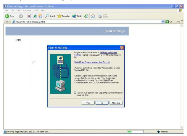
There are two settings for the Client site. One is "Media Option" for the User to determine if audio should be muted. The other is "Protocol Option" which allows choices on connection protocol between client and server. There are three protocol choices to optimize your usage - UDP, TCP and HTTP.
