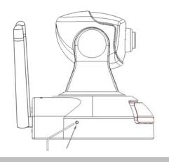
Restoring the factory defaults will erase any previous settings. Reset or restore the system after power on.
