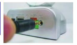
Attach the yellow RCA connector to the "Video" connector on your TV. Attach the white RCA connector to the "Audio" connector on your TV.
