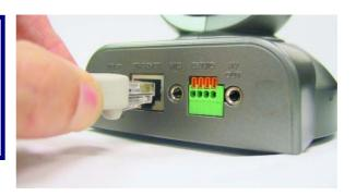
Please use a cross-over Ethernet cable if you connect this camera directly to a PC.
