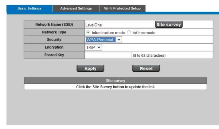
WPA supports two encryption methods, TKIP and AES, with dynamic encryption keys. Select the type of algorithm, TKIP or AES. The default is TKIP.
