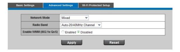
Network Mode - From this drop-down menu, you can select the wireless standards running on your network. If you have both Wireless-B, Wireless-G and Wireless-N (2.4GHz) devices in your network, keep the default setting, **Mixed**. If you have both Wireless-B, Wireless-G devices in your network, select **BG-Mixed**. If you have only Wireless-B devices, select **Wireless-B Only**. If you have only Wireless-N (2.4GHz) devices, select **Wireless-N Only**.
