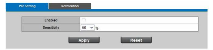
Enable PIR sensor to detect a moving infrared object such as a person in the dark. Sensitivity - is used to adjust the sensitivity of the PIR Sensor from 10 - 100%. The default sensitivity is 50%.
