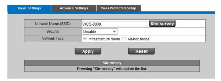
Network Name (SSID) - The SSID is the network name shared among all points in a wireless network. The SSID must be identical for all devices in the wireless network. It is case-sensitive and can be up to 32 characters in length. Make sure this setting is the same for all points in your wireless network.
