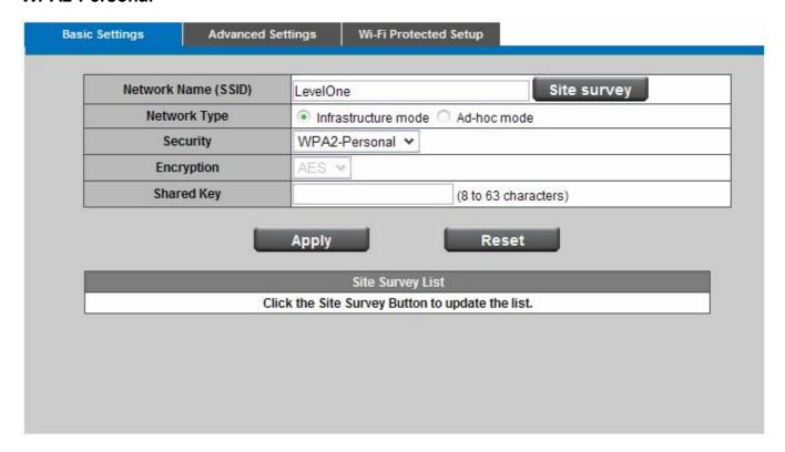
WPA2 supports AES encryption methods with dynamic encryption keys. Shared Key - Enter the key shared between the Router and the server keys. Enter a pass phrase of 8-63 characters.
