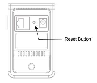
The reset button is used to reset the system or restore the factory default settings. Sometimes resetting the system can return the camera to normal operation. If the problems remain after reset, please restore the factory settings and install it again.
