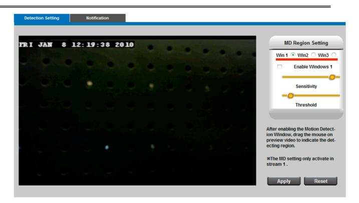
Detection Setting - Select and enable the motion detection windows function. Easier to
