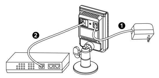
Please check your product package contains all the accessories listed in the foregoing Package Contents. Upon powering up, the power LED will become lighted first and then the device will go through booting process. The status LED will be steady amber for getting IP address. After getting IP Address, the link LED will blink orange while network connection is processing.
