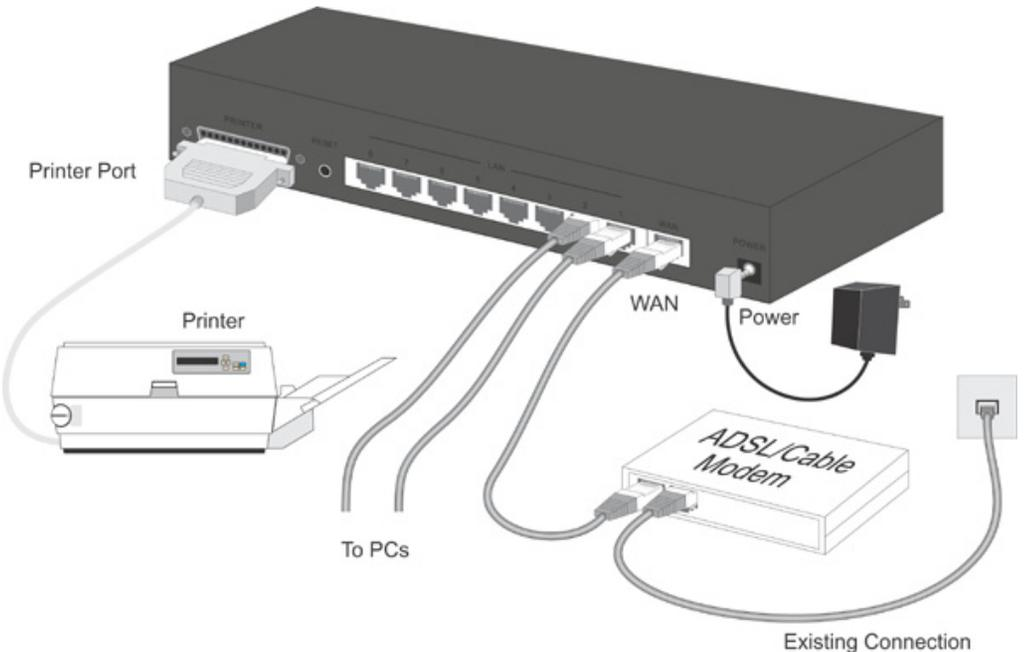
**Figure 4: Installation Diagram**
