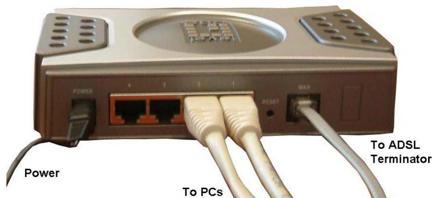
**Figure 4: Installation Diagram**
