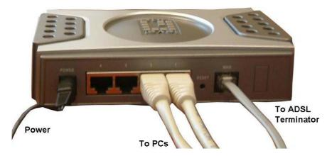
Figure 4: Installation Diagram
