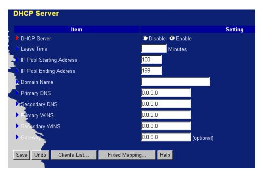
The settings of a TCP/IP environment include host IP, Subnet Mask, Gateway, and DNS configurations. It is not easy to manually configure all the computers and devices in your network. Fortunately, DHCP Server provides a rather simple approach to handle all these settings. This product supports the
