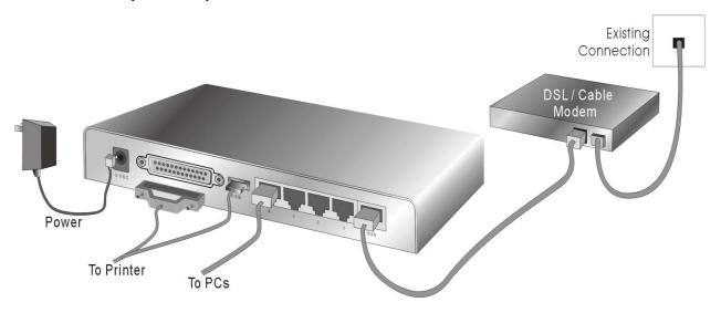
Figure 2-3 Setup of LAN and WAN connections for this product.
