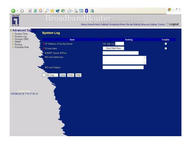
This page support two methods to export system logs to specific destination by means of syslog(UDP) and SMTP(TCP). The items you have to setup including:
