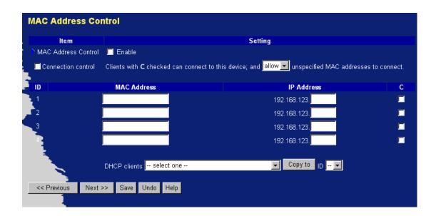
MAC Address Control allows you to assign different access right for different users and to assign a specific IP address to a certain MAC address.
