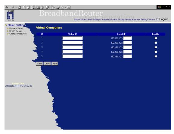
Virtual Computer enables you to use the original NAT feature, and allows you to setup the one-to-one mapping of multiple global IP address and local IP address.
