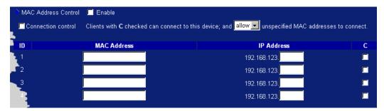
"Control table" is the table at the bottom of the "MAC Address Control" page. Each row of this table indicates the MAC address and the expected IP address mapping of a client. There are four columns in this table:
