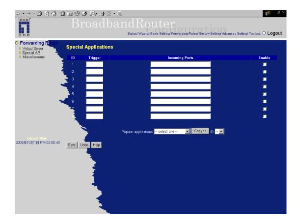
Some applications require multiple connections, like Internet games, Video conferencing, Internet telephony, etc. Because of the firewall function, these applications cannot work with a pure NAT router. The **Special Applications** feature allows some of these applications to work with this product. If the mechanism of Special Applications fails to make an application work, try setting your computer as the **DMZ** host instead.
