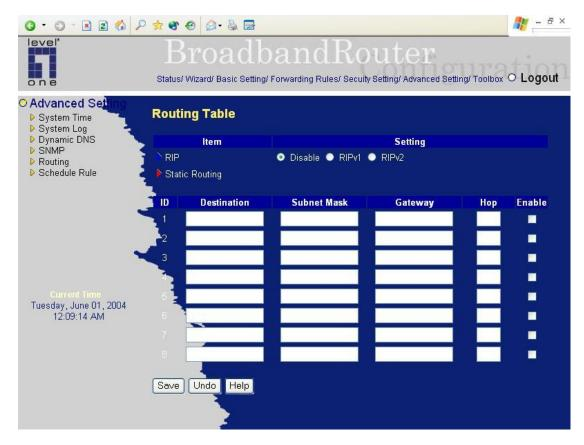
**Routing Tables** allow you to determine which physical interface address to use for outgoing IP data grams. If you have more than one routers and subnets, you will need to enable routing table to allow packets to find proper routing path and allow different subnets to communicate with each other.
