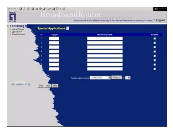
Some applications require multiple connections, like Internet games, Video conferencing, Internet telephony, etc. Because of the firewall function, these applications cannot work with a pure NAT router. The **Special Applications** feature allows some of these applications to work with this product. If the mechanism of *Special Applications* fails to make an application work, try setting your computer as the **DMZ** host instead.
