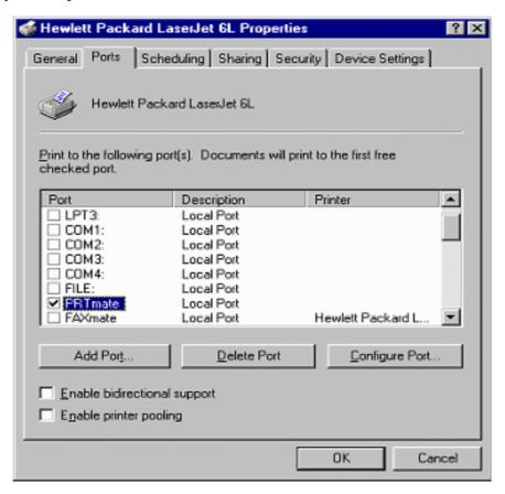
Compared to the procedure in last section, the selection of *Details* is equivalent to the selection of *Ports*, and *Port Settings* is equivalent to *Configure Port*.
