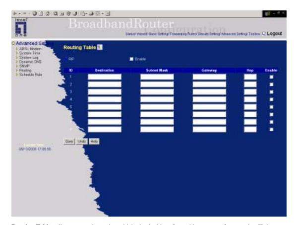
**Routing Tables** allow you to determine which physical interface address to use for outgoing IP data grams. If you have more than one routers and subnets, you will need to enable routing table to allow packets to find proper routing path and allow different subnets to communicate with each other.
