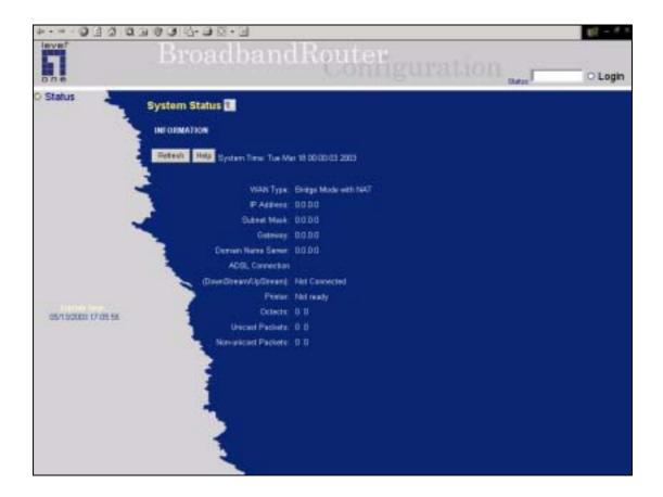
Activate your browser, and *disable the proxy* or *add the IP address of this product into the exceptions*. Then, type this product's IP address in the *Location* (for Netscape) or *Address* (for IE) field and press ENTER. For example: *http://192.168.123.254*.
