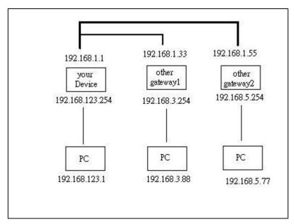
So if, for example, the host wanted to send an IP data gram to 192.168.3.88, it would use the above table to determine that it had to go via 192.168.1.33 (a gateway),
