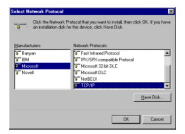
6. The TCP/IP protocol shall be listed in the Network window. Click *OK* to complete the install procedure and restart your PC to enable the TCP/IP protocol.
