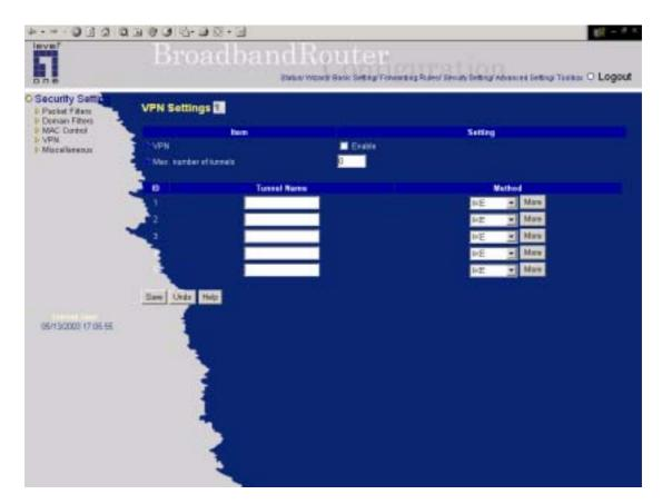
VPN Settings are settings that are used to create virtual private tunnels to remote VPN gateways. The tunnel technology supports data confidentiality, data origin authentication and data integrity of network information by utilizing encapsulation protocols, encryption algorithms, and hashing algorithms.
