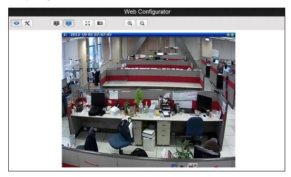
To capture the snapshots of the current live view, press the snapshot button. The snapshots are saved in Pictures folder.
