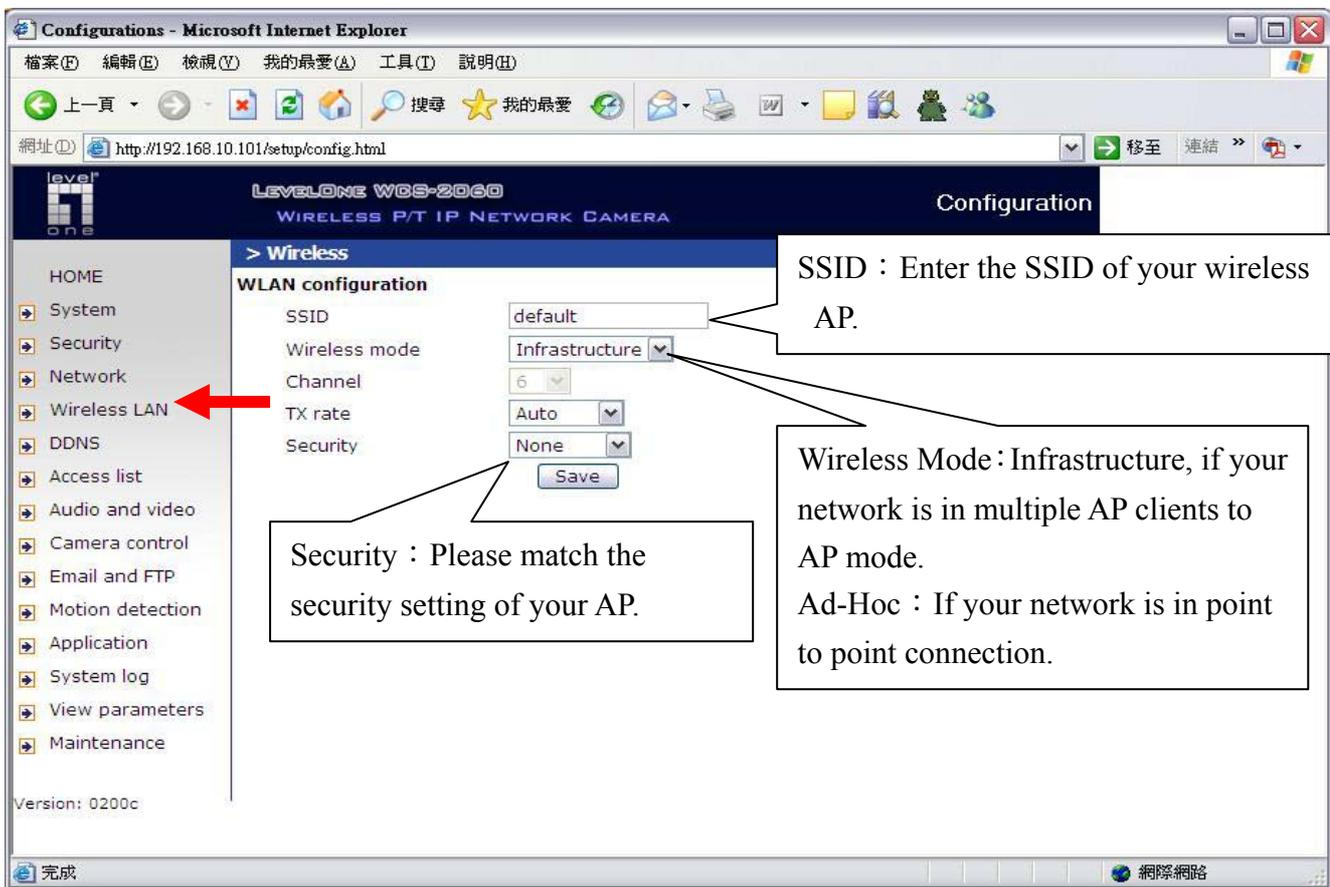
Please press "save" after configuration, and then unplug your power cord and RJ-45 LAN cable. Insert Power cord, do not insert RJ-45 LAN cable. LevelOne IP camera should automatically connect to the preset AP.
