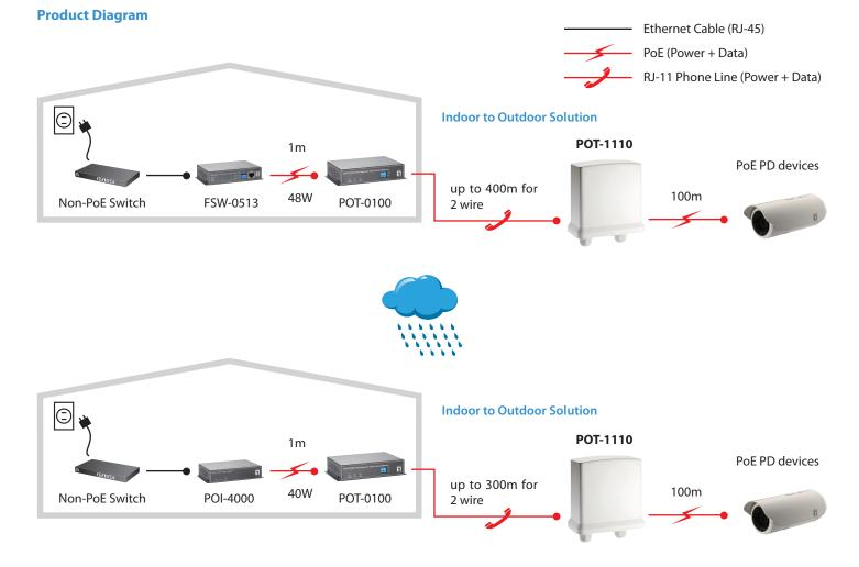
Note: These distances are typical results when used with 24AWG RJ-11 Cable
