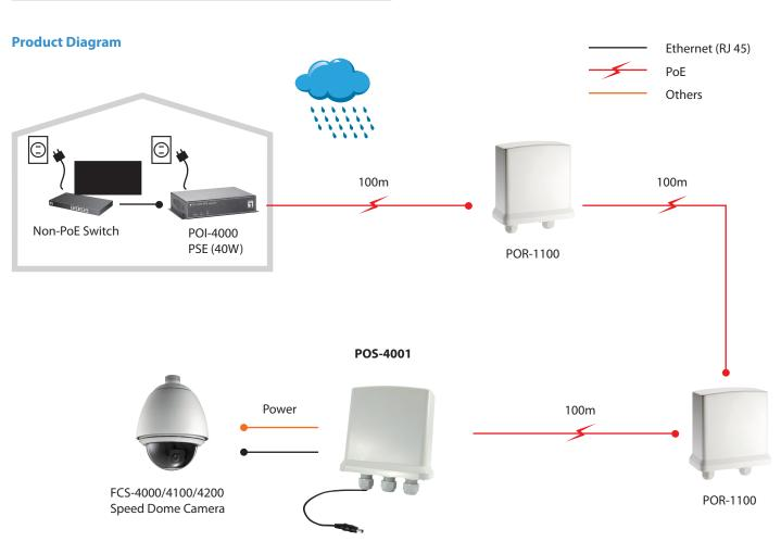
Note: These distances are typical results when used with 18~19 $\Omega$  24 AWG Cat.5 Cable
