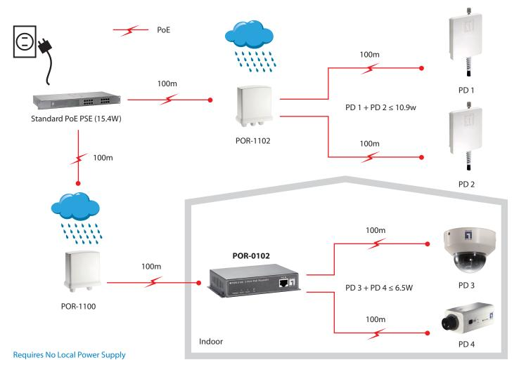
Note: These distances are typical results when used with  $18\sim19\Omega$  24 AWG Cat.5 Cable
