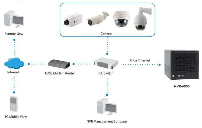
Order InformationNVR-4000: NVR Titan 4 Bay, 250Mbps, 4CH included, opt up to 64CH, Desktop CaseNVR-4000R: NVR Titan 4 Bay, 250Mbps, 4CH included, opt up to 64CH, 19 inch Rack MountNVR-4000-CH: Per cam license for NVR-4000 / NVR-4000R
