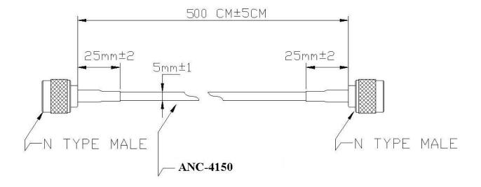
CABLE TYPE CFD 400 MODEL NO. ANC-4150 IMPEDANE  $50\Omega \pm 5\Omega$  LOSE <-2.0 dBi CABLE LENGTH 1M
