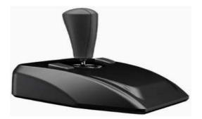
The CAS-4300 is USB Joystick designed for IP surveillance industry specifically. It has a three-axis joystick and USB interface. It integrates with CMS surveillance software for PTZ controls. You just connect the joystick to the USB port on your computer and control the PTZ cameras.
