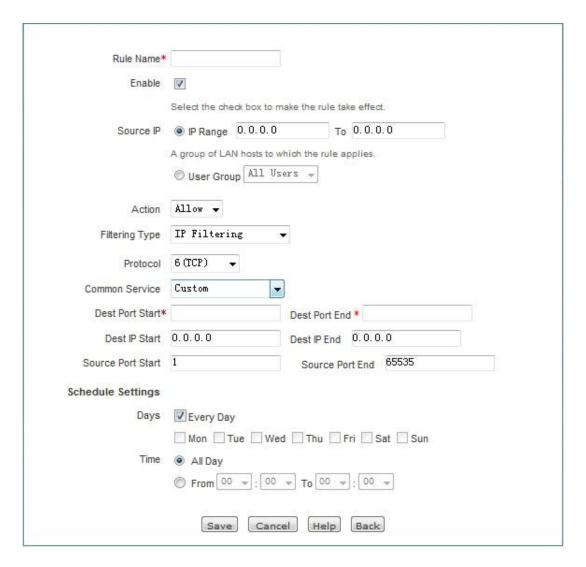
Figure 12\_4 Access Control Settings - IP address filtering
