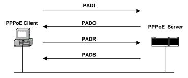
Figure 9\_9 Basic workflow of Discovery stage
