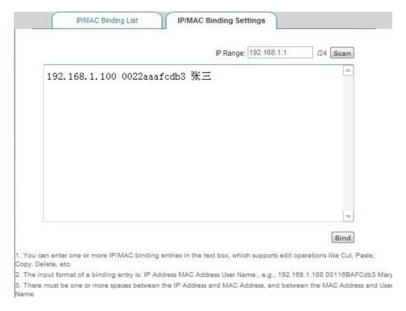
Figure 9\_5 IP/MAC binding configuration
