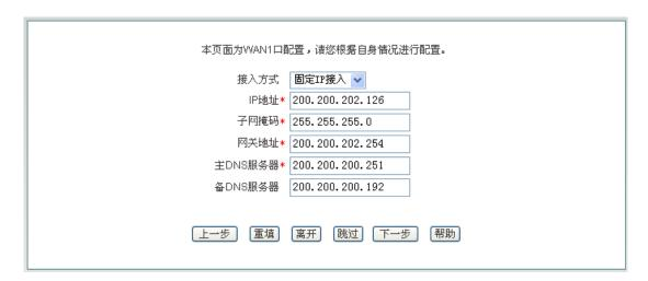
Figure 4-3 Configuration Wizard - Static IP access
