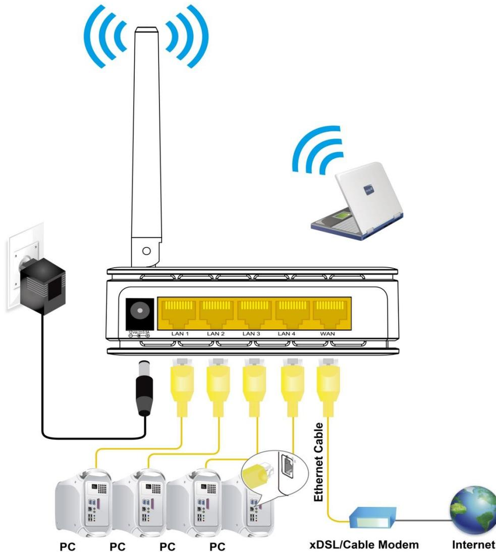
Figure 4: Overview of Hardware Connections
