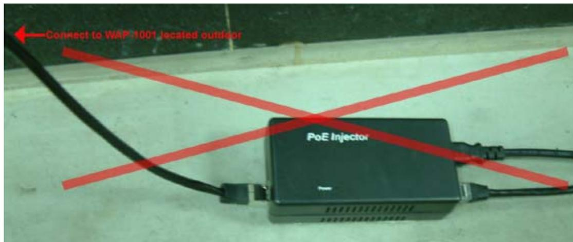
When placing WAP-1001 in outdoor environment, there is an Ethernet cable connecting WAP-1001 and POE Injector. If place the POE injector on the ground like the photo shown, rain or dust might leak via the Ethernet cable and permeate into the POE injector. This will result in power failure.
