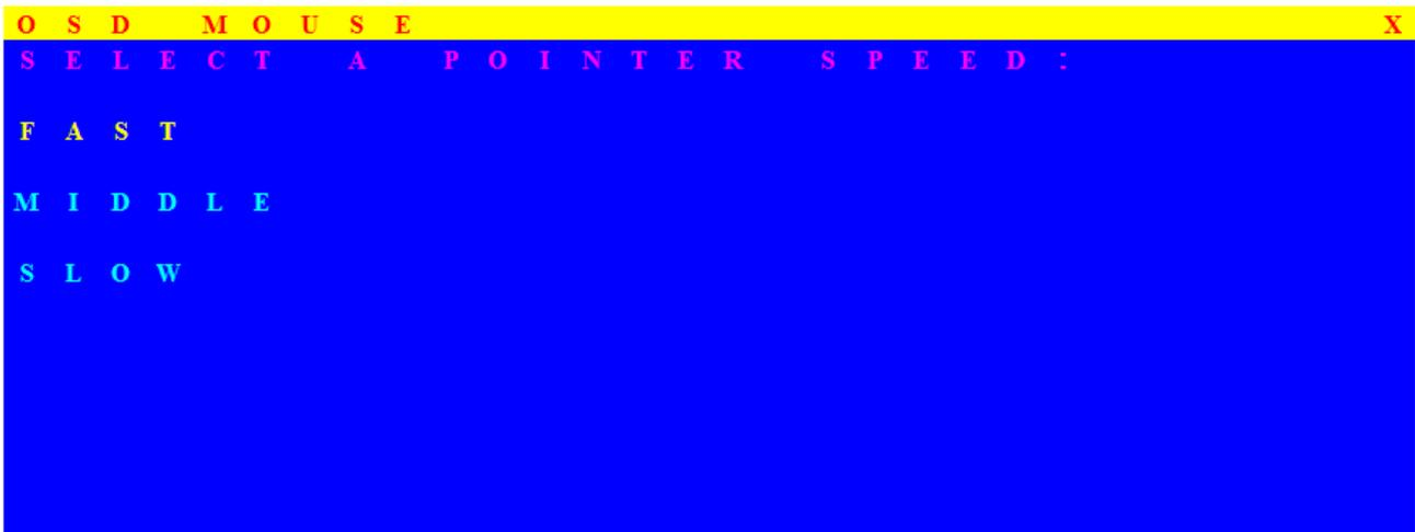
You can change the moving speed of mouse cursor in this item. There are three levels to choose from. The fastest moving speed is “FAST”, the second is “MIDDLE” and the slowest is “SLOW”.
