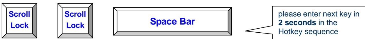
**Example #2** – To switch to Bank 1 Port1, press “**Scroll Lock**”, “**Scroll Lock**”, and “**1**”, “**0**”, “**1**”.
