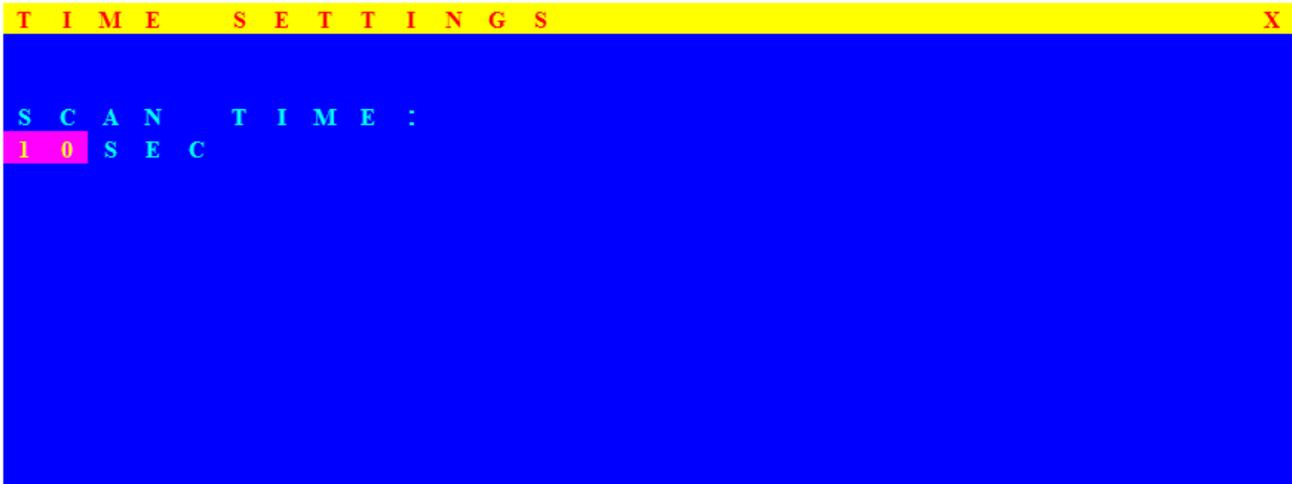
When the Auto-Scan function is activated, the KVM switch will auto-scan the host ports one by one in the interval as setting. Notice that the port without connecting to a computer/server will be skipped over on the scan. The interval range is 5 ~ 99 seconds, and the default interval is 10 seconds. Press “**Enter**” key to save the SCAN TIME setting.
