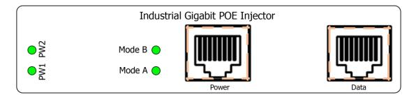
Mode A Green LED ON --For End-Span POE power 1,2,3,6
