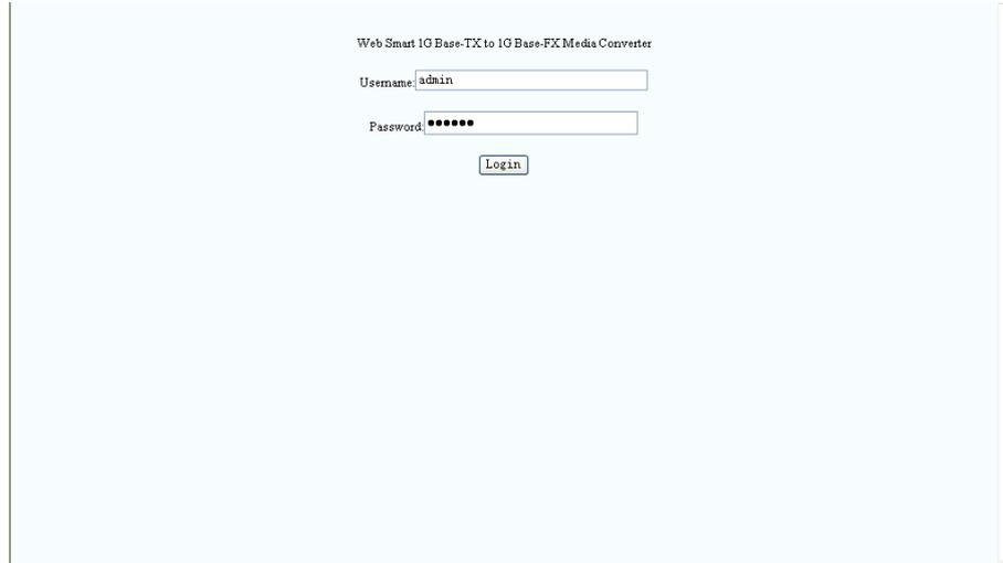
We must input the correct the password to login the web, otherwise we could not access any web pages. The default Username is admin and the default password is 123456 and could be changed in the web. If we don't have any operations in 15 minutes, we need login again.
