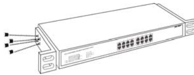
Figure 1. Combine GSW-1674T/2474T with the provided screws
