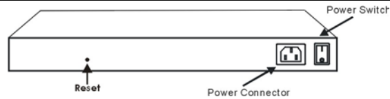
Figure 5. Rear panel of the Switch
