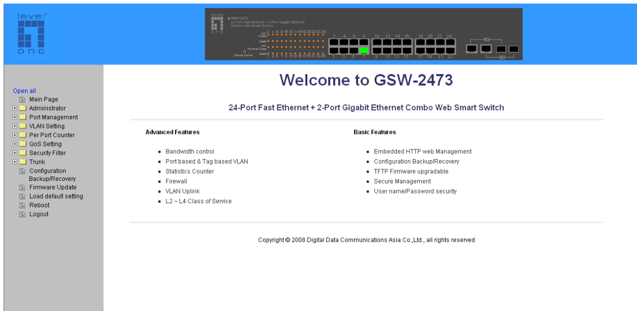
Main Page of 24-Port Fast Ethernet + 2-Port Gigabit Ethernet Combo Web Smart Switch
