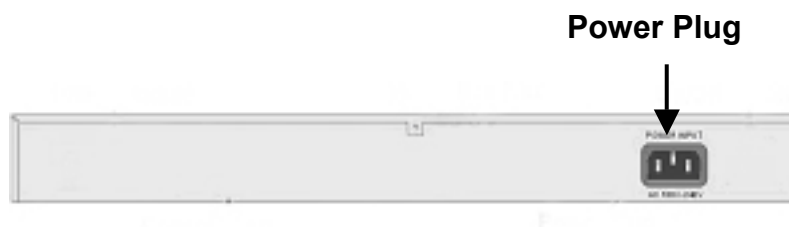
Figure 2-3. The Rear Panel of the LevelOne GSW-2470TGX Smart Switch
