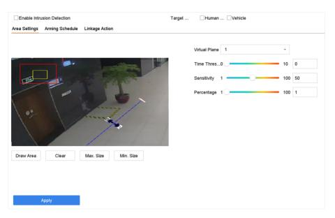
**Figure 6-7 Line Crossing Detection**
