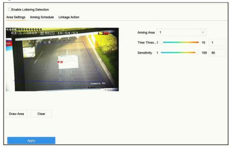
Figure 6-11 Loitering Detection
