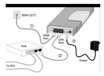
Note: The Level One ISDN Router incorporates a DHCP Server. If your LAN already has a DHCP Server, set DIP switch 2 ON to disable the ISDN Router's DHCP Server.
