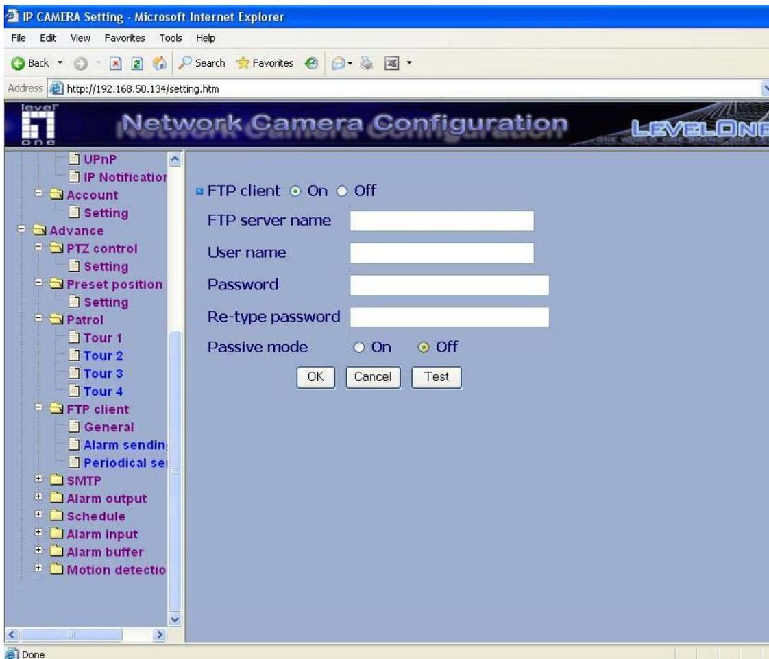
**FTP client function** : To activate the FTP client function, select **On**. The FTP client setting page appears. When you do not wish to use the FTP client function, select **Off**.
