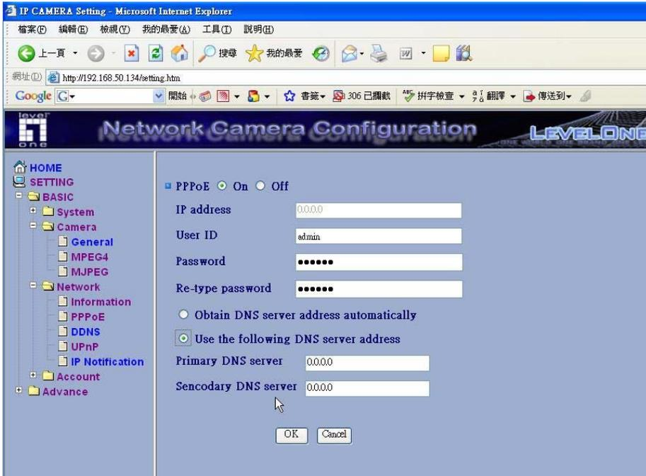
**IP address** : The IP address obtained at the PPPoE connecting with network.
